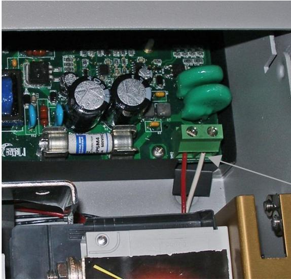
**Step 7:** Strip one end on the red and white wires included in the kit  $\frac{1}{4}$ " and connect them as shown with the red wire on the left side of the terminal block marked "PV+" and the white wire on the right side marked "PV-". Route the wires downward under the large switch.
