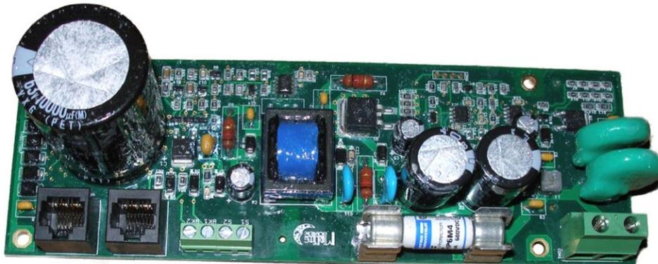
When using the Birdhouse with any one of the Disco combiners you must also add the **MNDiscoPSB** Power Supply Board. The Power Supply Board is already incorporated into the Arc Fault combiners. The Power Supply Board does not need to be added when using the Birdhouse with Arc Fault combiners or an external power supply.
