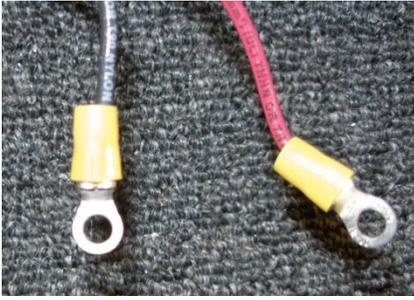
Ring lugs are included to allow easy installation of the MNSPD. If they are to be used, then you would need to strip the wire, push it into the barrel of the ring lug and crimp the barrel with an appropriate crimper. Make sure to pull on the wire after crimping to verify that the crimp is adequate.
