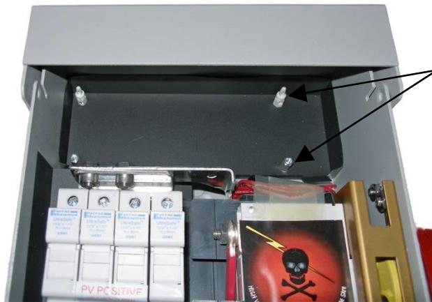
**Step 3:** Install metal standoffs (2) and plastic PCB supports (2).
