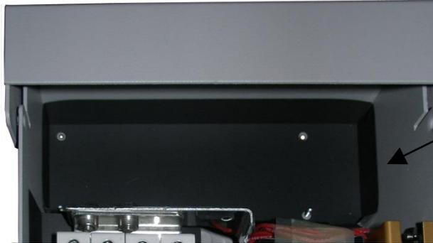
**Step 2:** Place the Formex insulator as shown.
