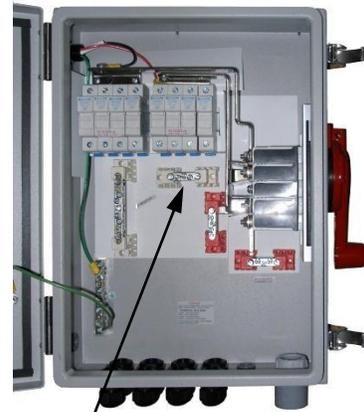
Install block. Refer to torque chart on page 4. Use screws removed in step 1
